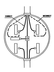
METER SOCKET WIRING (3 WIRE SERVICE)
